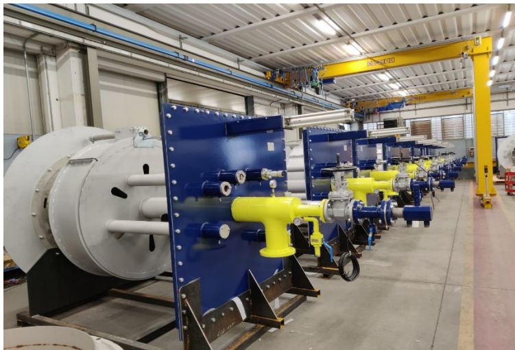
Unit 5 natural gas burners post fabrication at factory
