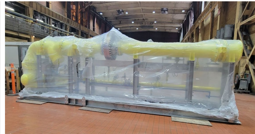
Unit 5 control valve skid and piping run for conversion staged at North Omaha Station
