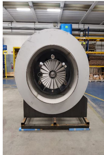
Unit 5 natural gas burners post fabrication at factory
