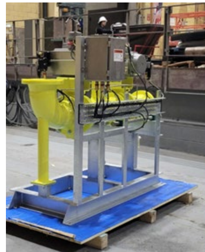
Unit 5 control valve skid and piping run for conversion staged at North Omaha Station
